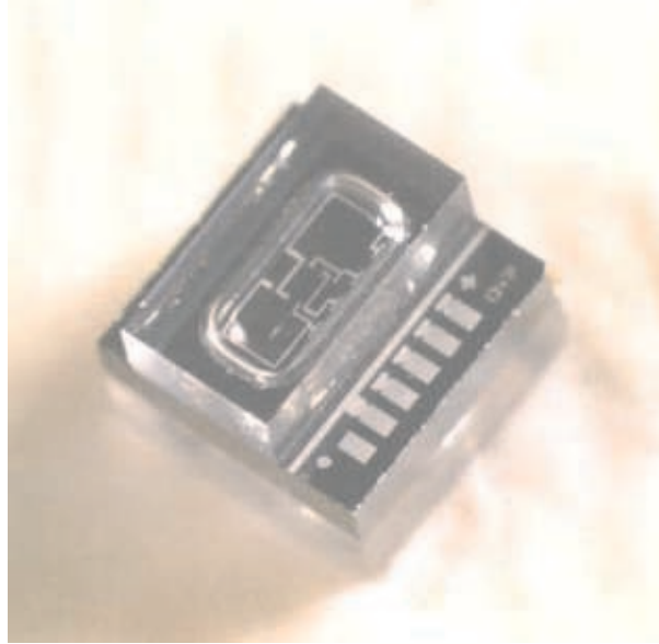
Figure 3.23: Silicon pressure sensor SP15 bonded with glass cover (Courtesy Sensor AS - An Infineon Technologies Company).
