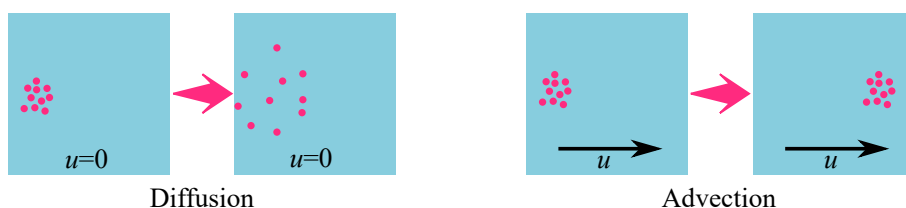
Figure 4.17: Motion of particle in a fluid induced by only diffusion (left) or by only advection (right).
